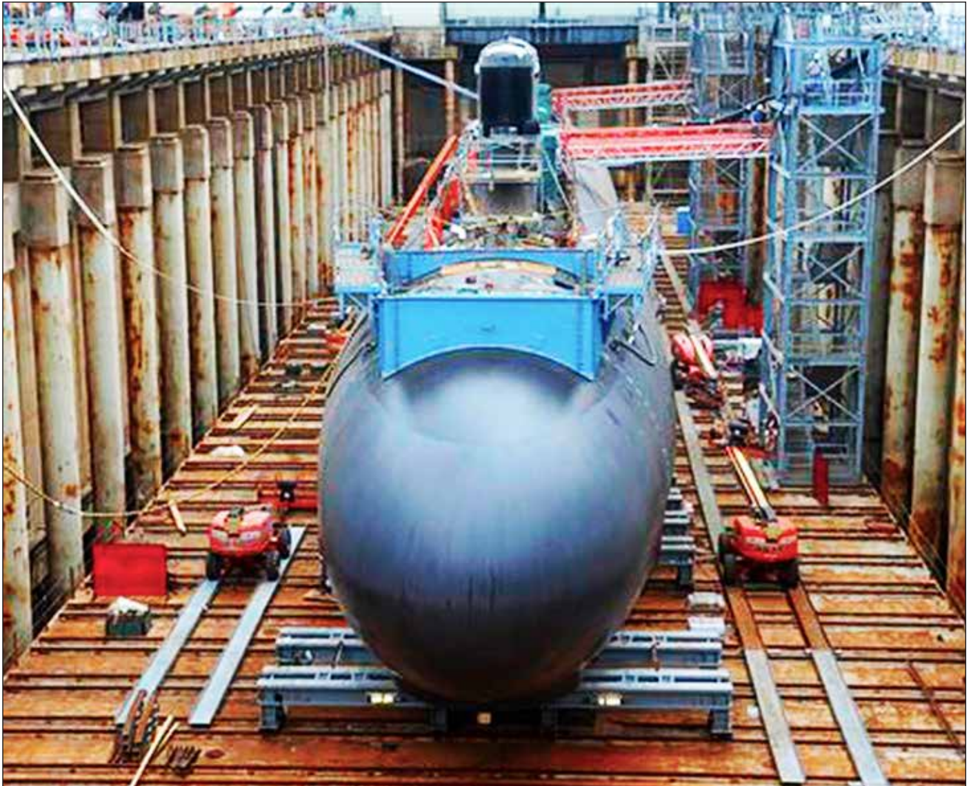
In this July 30, 2015 photo, shipyard workers at General Dynamics Electric Boat prepare the submarine Illinois for float-off in Groton, Conn. The U.S. Navy is using a new painting process and dozens of other innovations aimed at reducing the maintenance needs for attack submarines, which are coming out of service faster than they can be replaced. (Jessica Hill/AP.)
